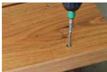
Step 2: Fasten with SPAX-BIT T-STAR plus T40.
